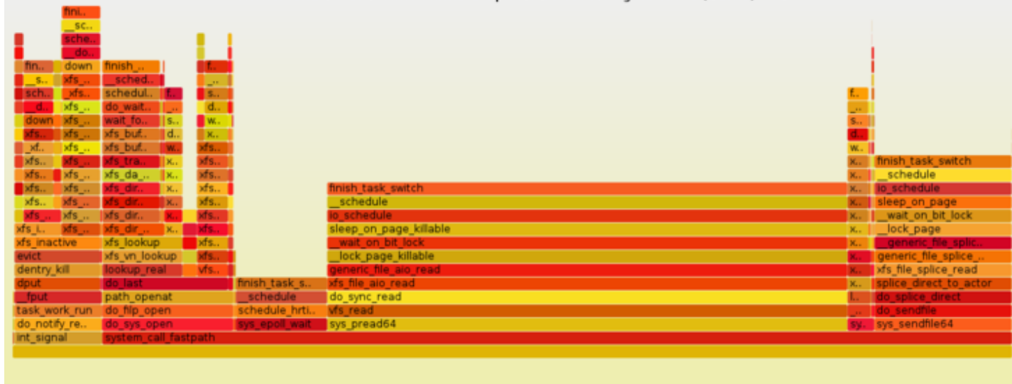
Kernel-land off-CPU Time Flame Graph for 20 sec for nginx-cache (16m3) - V1
